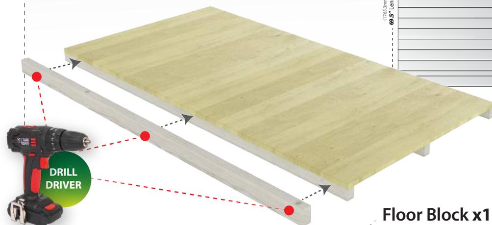
● = Drill Points using screws provided as shown
