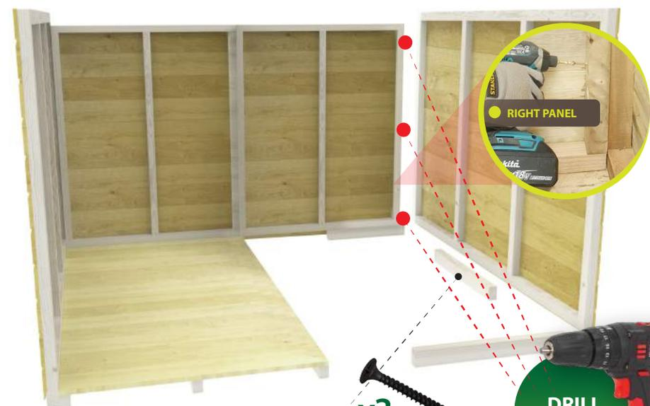
Using the Floor Block Posts, elevate the right side panel and screw in sides to secure againsts the 2nd back panel side post as shown.
