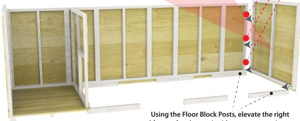
Using the Floor Block Posts, elevate the right side panel and screw in sides to secure againsts the last back panel side post as shown.
