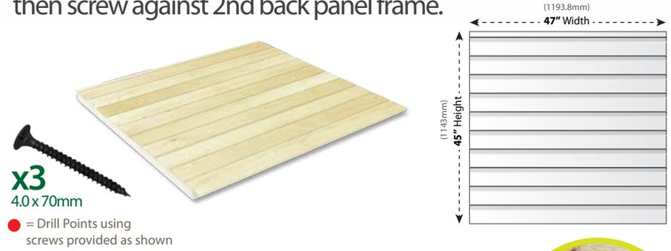
Position the 3rd back panel in place as shown on diagram below. Use Floor Blocks to elevate. The back panel must be the same height as the 1st and 2nd back panel which is 63mm from the ground.
