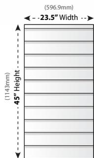
Position the 2nd back panel in place as shown on diagram below. The back panel 2 must be the same height as the 1st back panel which is 63mm from the ground to back panel frame bottom.
