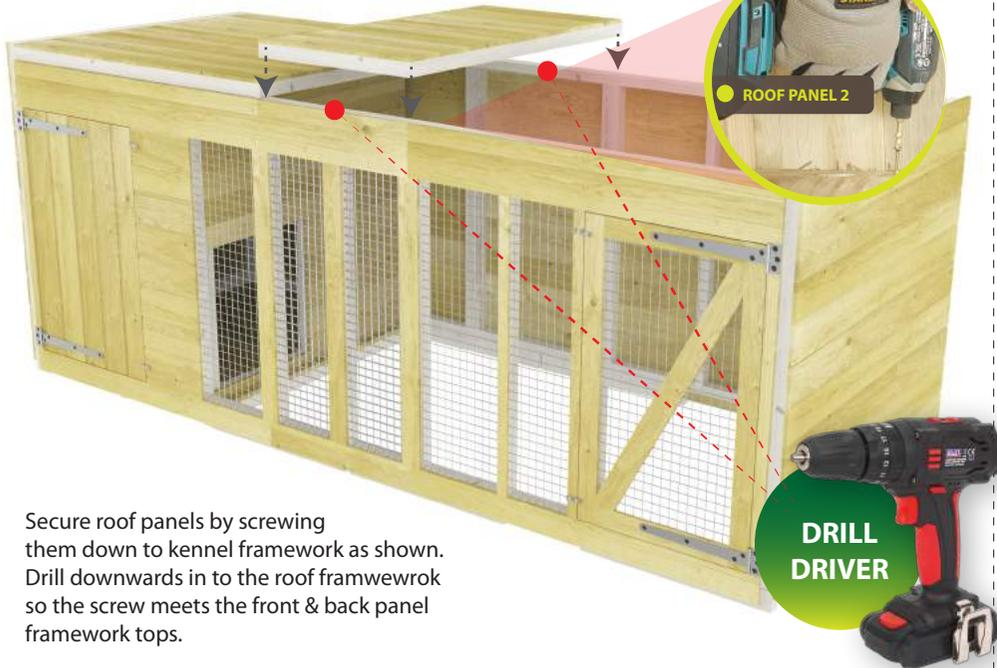
Secure roof panels by screwing them down to kennel framework as shown. Drill downwards in to the roof framewrok so the screw meets the front & back panel framework tops.
