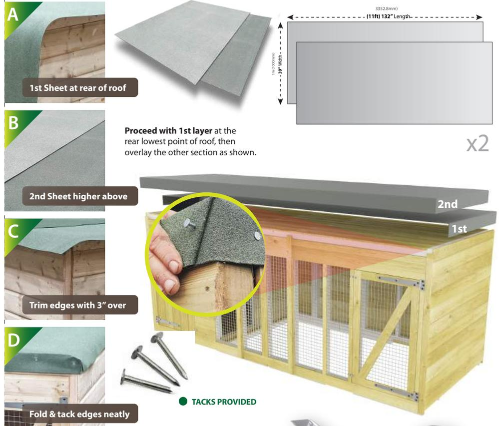
After cutting away the excess felt, neatly fold over the edges and secure each section down by tacking them to the kennel sides. **PROTECT YOUR KENNEL AGAINST THE RAIN & ELEMENTS.**
