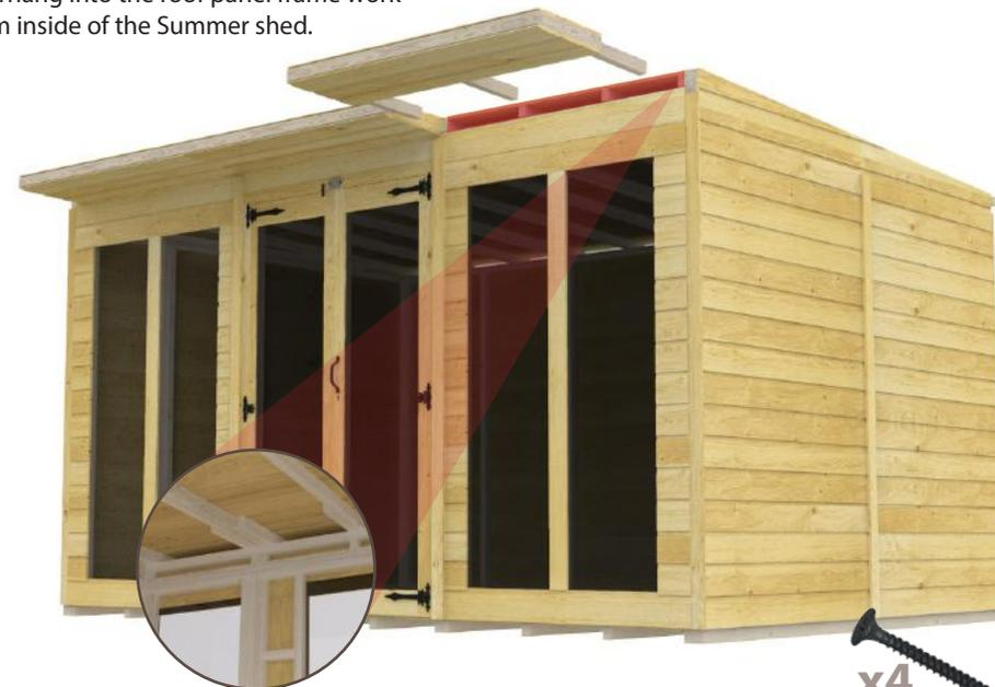
● = Drill Points using screws provided as shown
