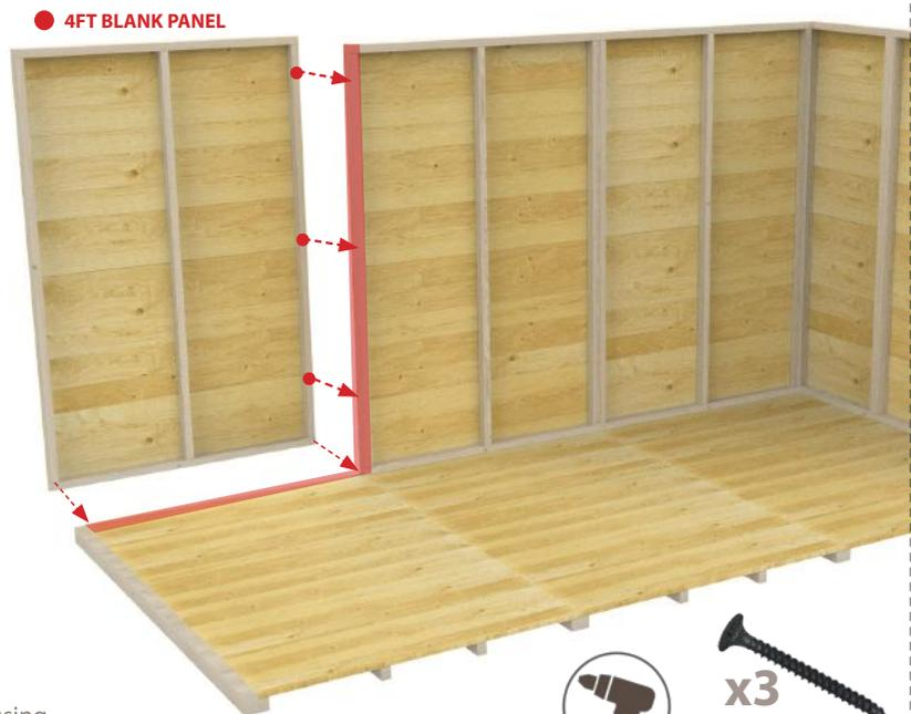
● = Drill Points using screws provided as shown
