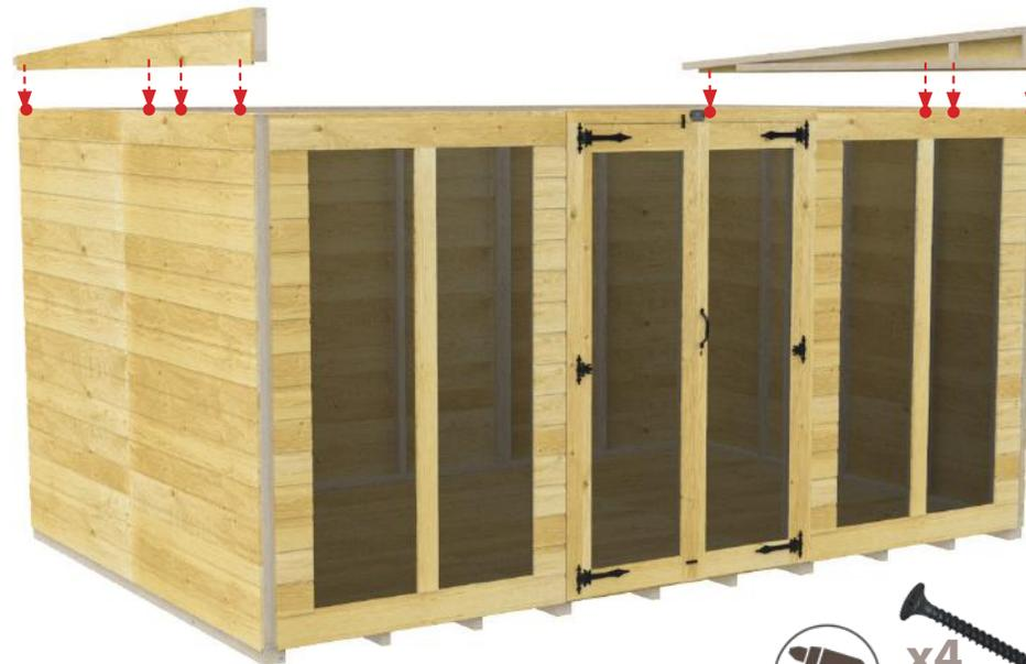
● = Drill Points using screws provided as shown
