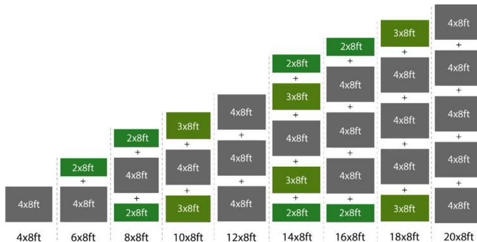
This process will be the same for any build this has a depth of 8ft. The 8ft will be constructed using two 4ft sections.
