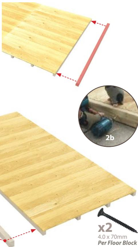
● = Drill Points using screws provided as shown
