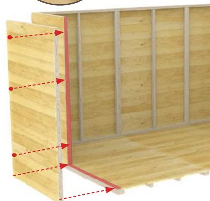
● = Drill Points using screws provided as shown
