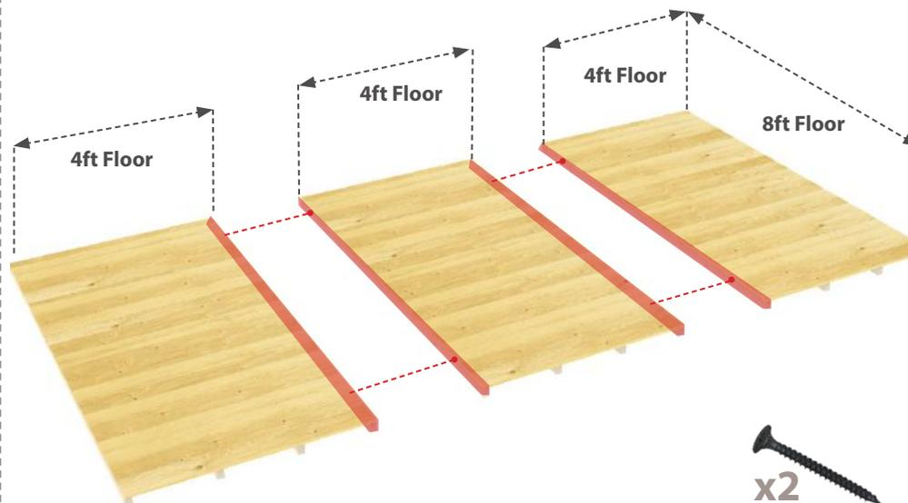
● = Drill Points using screws provided as shown
