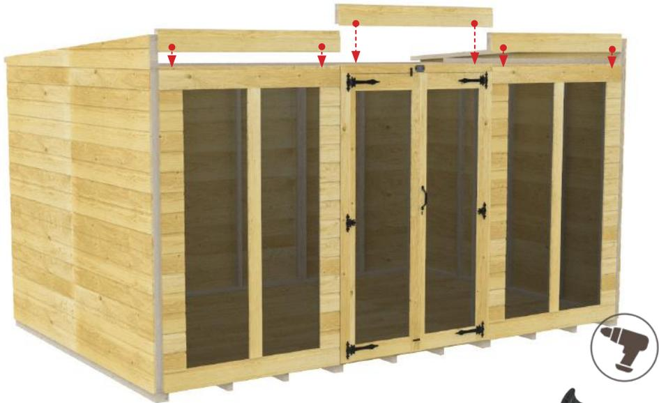
**12c.** Attach the sections down by screwing through the inner framework of both panels.
