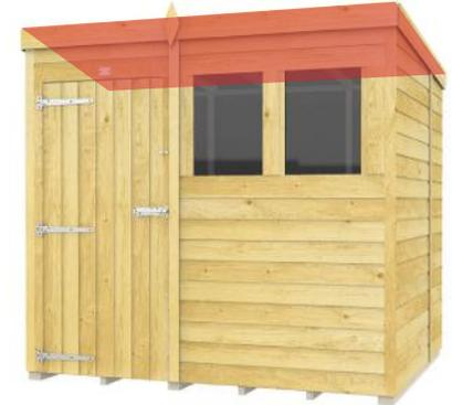
**15a.** Apply the roof felt as shown. Apply lower levels first to create correct rain run off positions.
