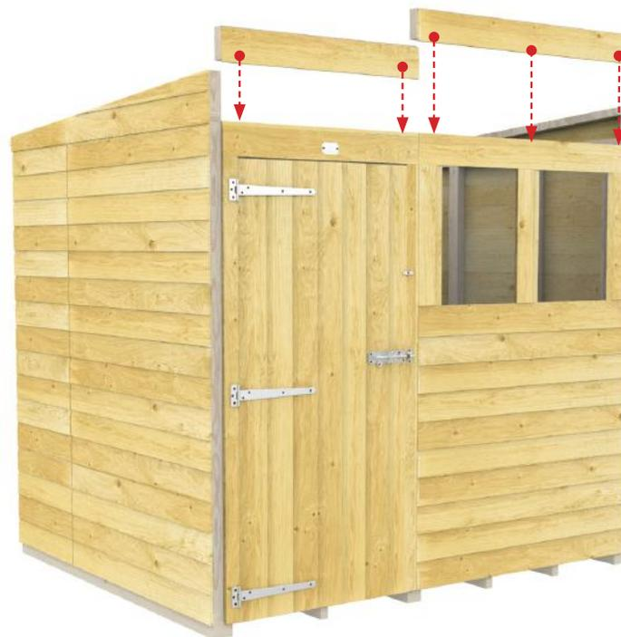
**11c.** Attach the sections down by screwing through the inner framework of both panels.
