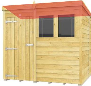
**14a.** Use the Stanley knife to cut your felt into the correct size. Using the table below, find the **Build** size that you have and cut your felt down to achieve the size that you will need.
