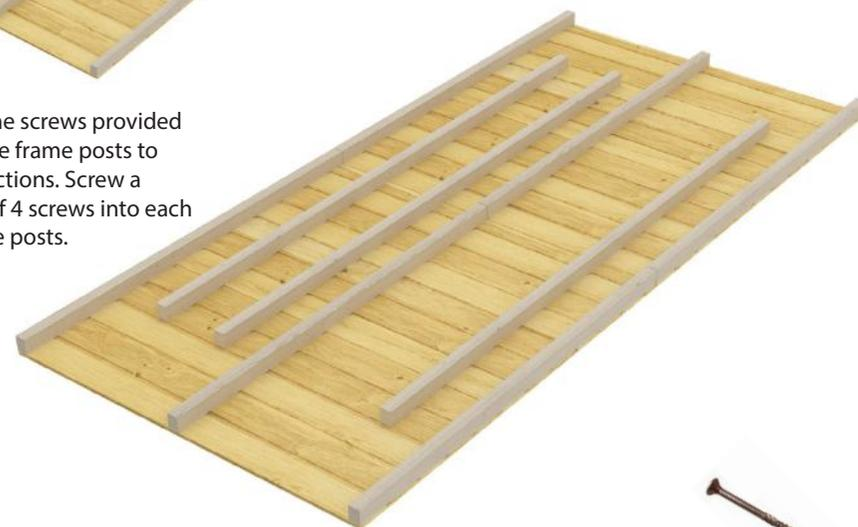
**REMEMBER** Do not screw the 100mm screws all the way through, just enough for the frame post and post to attach.
