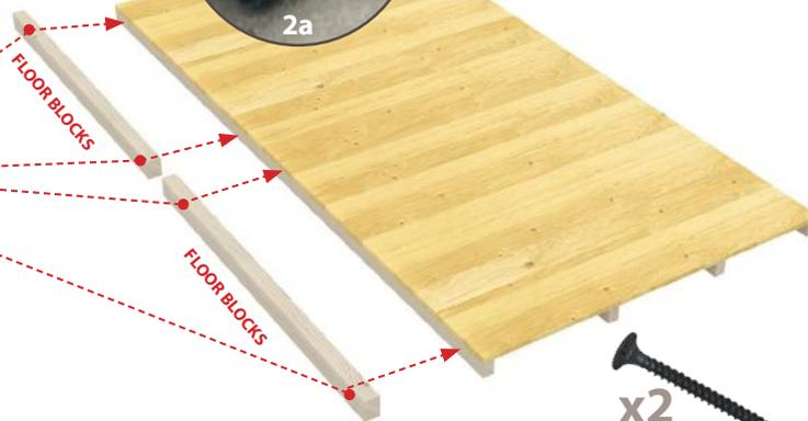
● = Drill Points using screws provided as shown
