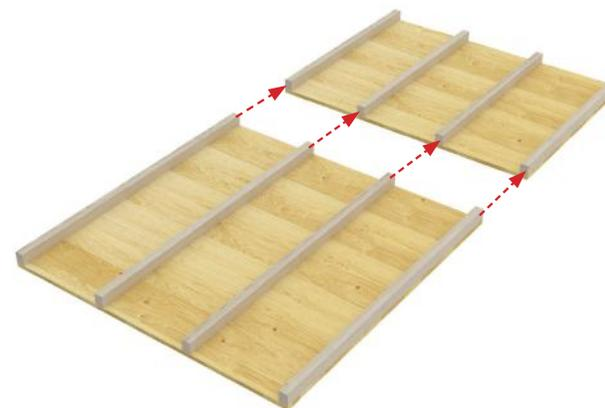
This process will be the same for any build this has a depth of 7ft. The 7ft will be constructed using one 4ft section and a 3ft section.
