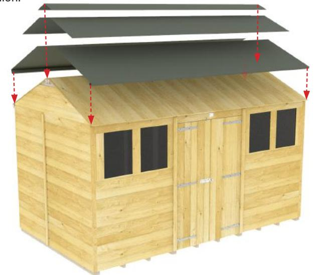
**15c.** Trim down excess felt with a stanley knife. Remember to overlay the 1st felt to avoid rain leaks.
