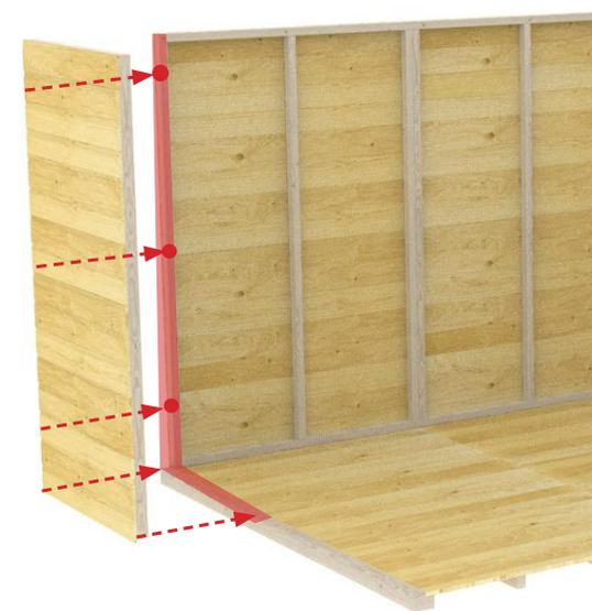
**7b.** Repeat this step until all Side Panels have been secured in place using three screws.
