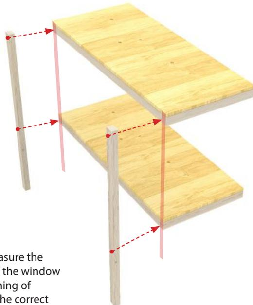
**18b.** Once the top panel is in place, measure the distance of the framing on the inside of the window panel from the above to the below framing of the bottom window. This will give you the correct placement of the second Shelf Panel. (About 10cm from the bottom frame post).
