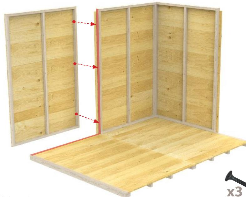
● = Drill Points using screws provided as shown
