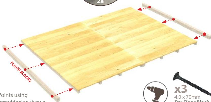
● = Drill Points using screws provided as shown
