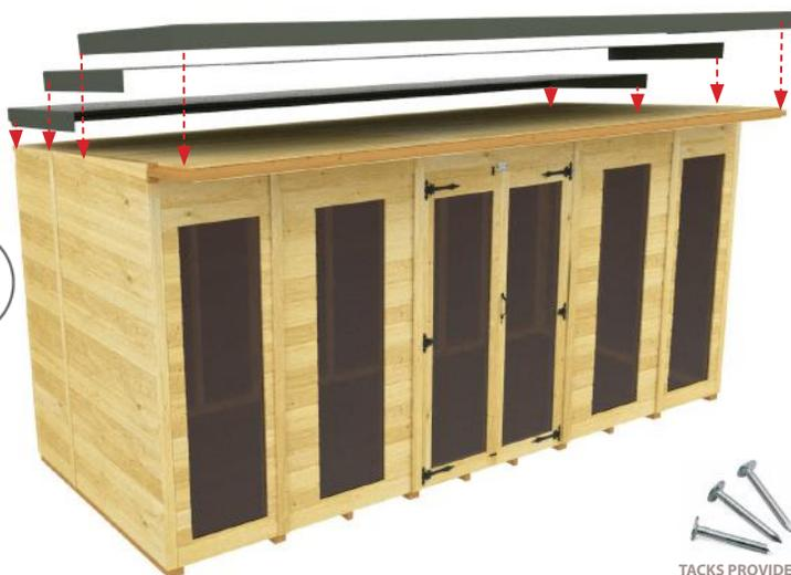
**20c.** Trim down excess felt with a stanley knife. Remember to overlay the 1st felt to avoid rain leaks.
