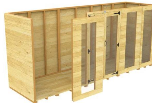
**9a.** Place the final front panel as shown (Below) to complete the outer framework. Then adjust and screw down the panels to the shed floor to make the build secure. This requires an extra 3x Screws.
