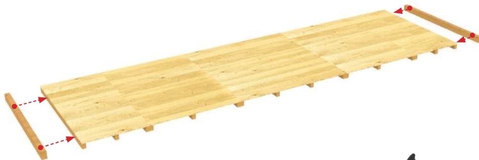
● = Drill Points using screws provided as shown
